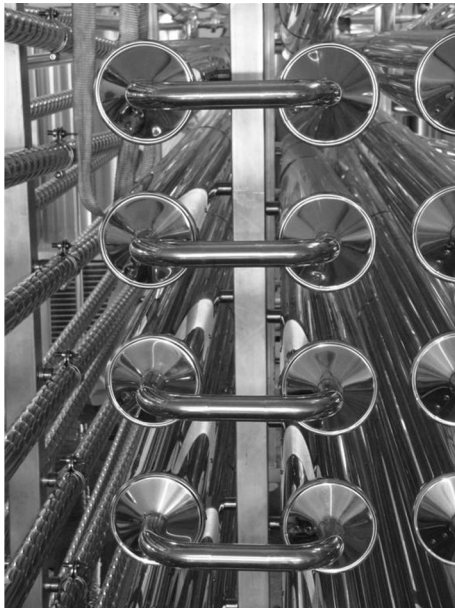
The ViscoLine tubular heat exchanger connected in series with insulation.
