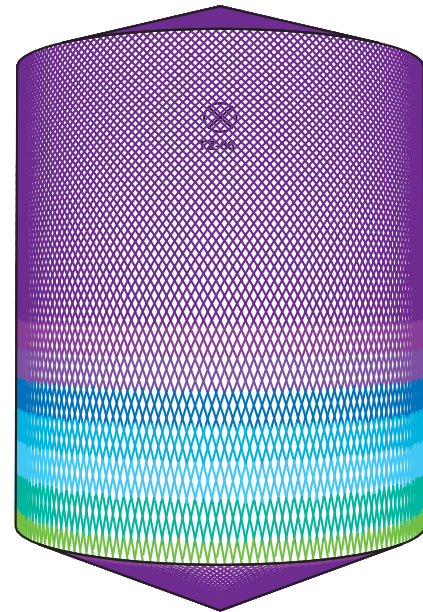
D8m H10m, Toftejorg TZ-66, 4 x ø10 mm, 0% Time = 23.3 min., Water consumption = 10868 l
