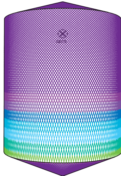
D8m H10m, Toftejorg TZ-79, 4 x ø10 mm, 0 % Time = 23.3 min., Water consumption = 10868 l
